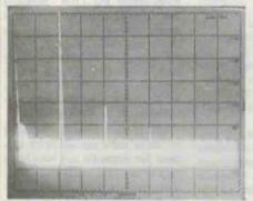
Figure 2. Same 10 MHz signal on the spectrum analyser shows that signal, thought to be a pure sine wave, has harmonics. Analyser dispersion is set at 5 MHz/div and shows first and second harmonics at 20 and 40 MHz. The fundamental (10 MHz) is set to top of screen and the relative amplitudes of the harmonics, referenced to the signal are seen to be 40 dB and 50 dB below the signal.
