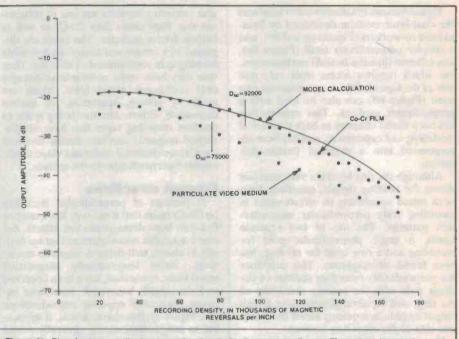
Figure 8b. Plot of output amplitude v recording density for the same medium as Figure 8a, with an advanced video head with a small gap (10.5u").
