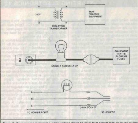
Figure 3. Mains power consideration. Lamp wattage should be equal to or greater than, up to two or three times, that of the equipment being serviced.
