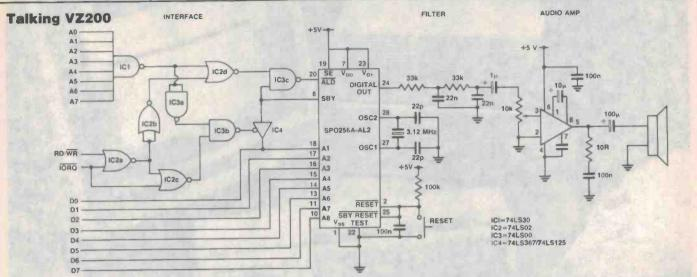
Matthew Bennets of Corowa NSW, sent us this circuit designed to allow speech processing from the VZ200 computer. You could adapt the idea to any computer where you can control seven address and seven data lines, plus two control lines.
