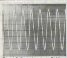
Figure 1. Oscilloscope trace showing 10 MHz signal. If you expect this to be a pure sine wave then see Figure 2.
