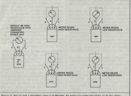
Figure 2. How to test a transistor using a multimeter. An analogue meter should be on its low ohms range. Note that the polarity of the meter will reverse; the black lead (---) becomes the positive potential. Digital meters should be on 'diode' test without reversed lead polarity.
