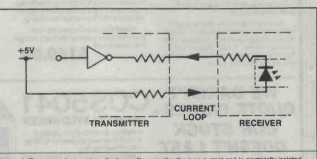
Figure 1. The current loop system; the transmitter provides the loop current and is electrically isolated to obviate loops that can cause earth hum.
